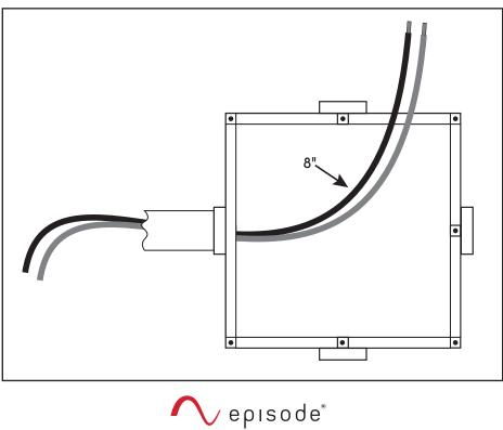
**Pro Tip**: Make sure that all PVC connections are securely glued. Use silicone caulk to seal any openings used for cable. Allow caulk and glue to dry completely before burying the box.
