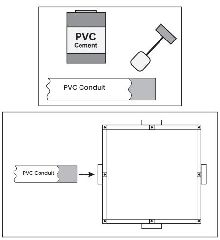
3. Route the cable through the conduit and pull at least 8 inches (200mm) of cable into the box cavity.
