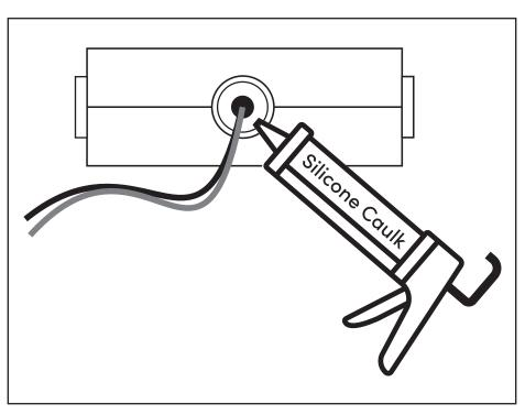
**Pro Tip**: Make sure that all PVC connections are securely glued. Use silicone caulk to seal any openings used for cable. Allow caulk and glue to dry completely before burying the box.
