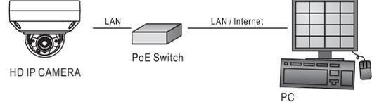
(3) Use PoE power injector and the network switch connected to the network.
