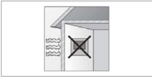
Fig. 7: Installation site - Exterior wall
