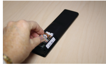
Figure 2. Remove Old Batteries
