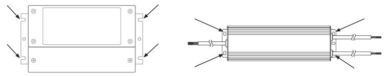
The 30W, 60W, and 96W power supplies have a wiring enclosure with line voltage and low voltage wiring compartments with knockouts that can be used to safely run your wiring. For the 200W and 300W power supplies, install your high voltage wiring inside an approved wallbox or enclosure. Ensure that all wiring complies with local electrical codes and regulations.
