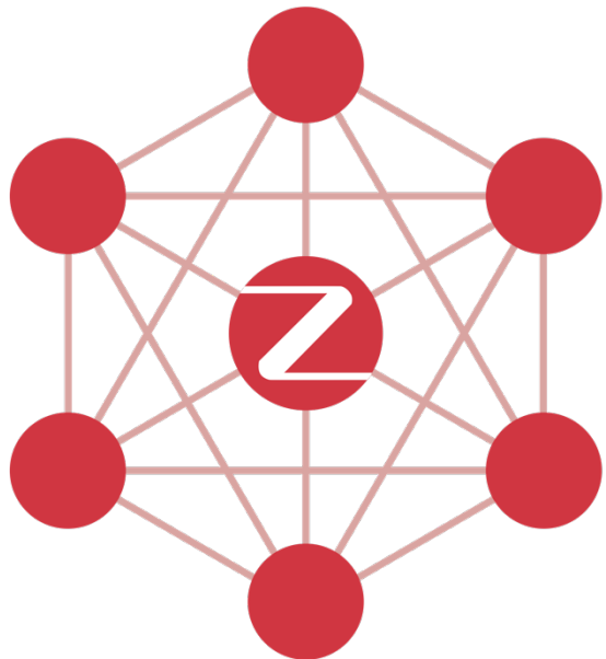
Mesh network topology (Zigbee)
