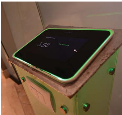
Each meeting room has its own pedestal that glows green if available and red when occupied.
